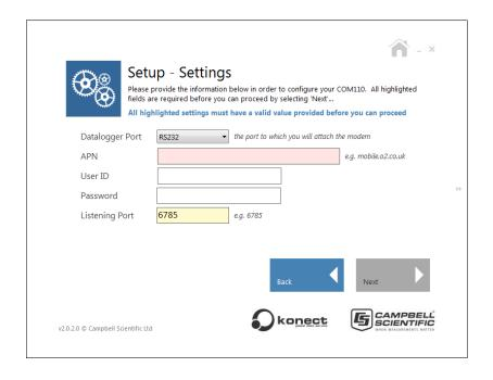
This screen varies with logger type. A datalogger port option will be shown if different connections are possible so you can select the port on the logger the COM110A will be connect to using the drop down option list. Select RS232
