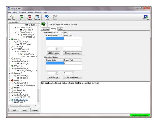
You then need to attach a datalogger entry to the PakbusTCPServer for each datalogger in your GPRS network, making sure each logger has a unique Pakbus address which matches the logger Pakbus address set in the logger using the Device Configuration program. Other settings, such as data collection parameters, clock correction are set as normal in the datalogger tabs.
