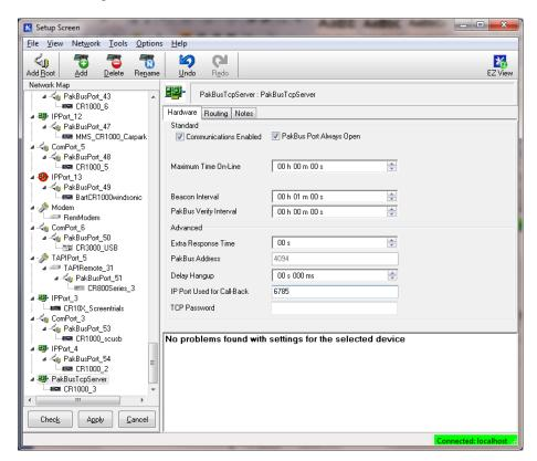
The details of the way calls are routed via this port are entered in the routing tab as shown below and fully documented in the Loggernet help system. If you are able to call out to a device that has a fixed IP address enter it in the Outbound Pakbus connection table, matching the logger Pakbus address to its fixed IP address, with the logger's Pakbus service port appended to the end.
