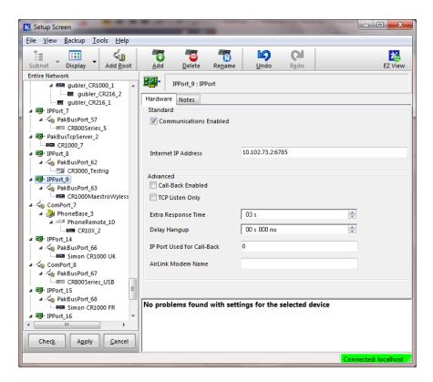
Where the number of outgoing IP ports is limited, perhaps due to a firewall restriction, Pakbus loggers with discreet Pakbus addresses can be connected via a PakbusTCPServer, as shown below (Loggernet 4 onwards). The IP address of the remote logger is entered in the Routing screen as an Outgoing connection.
