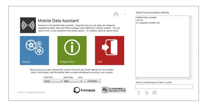
When this window is opened on the home screen an additional entry window appears below the activity window that lets you send commands directly to the modem. This can be used to send diagnostic commands to the modem and also to send non-standard configuration commands. Prior to using this make sure the COM port and baud rate are selected correctly to match the connection and setup of the modem.
