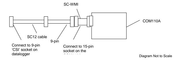
Figure 1 Connecting the COM110A modem to a Datalogger
